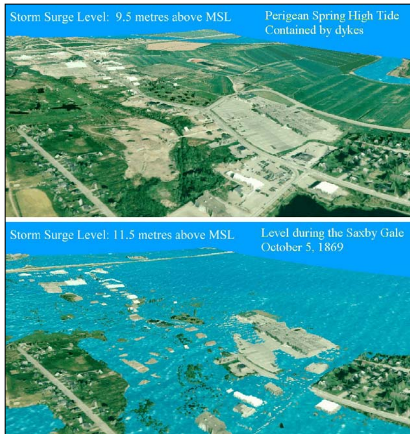
Figure 2. Example of flood-risk maps for the Truro area simulating the Saxby Gale storm surge. A perspective view of air photos draped over the LiDAR digital surface model (DSM) for lower Truro. Top image represents the water level extent simulated from the LiDAR at perigean high tide. The lower image represents the water level from the Saxby Gale event of 1869 draped over the air photo and LiDAR DSM.
