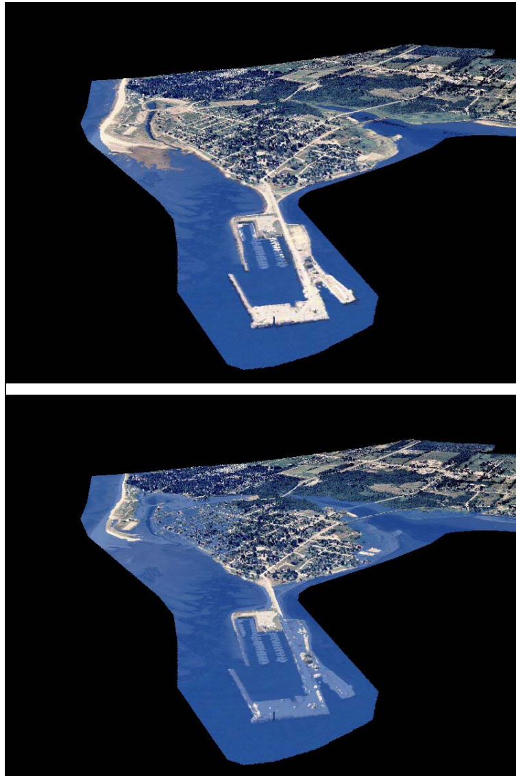
Figure 6. Perspective view of air photographs draped over the LiDAR digital surface model (DSM) for the Pte-du-Chêne area along the New Brunswick coast of the Northumberland Strait. The upper image represents mean water level. The lower image represents the water level of the January 2000 storm simulated using the LiDAR DEM (air photos courtesy of Services New Brunswick).
