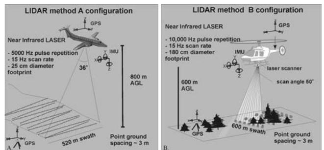
**Figure 2** A LIDAR configuration for acquisition method A.
