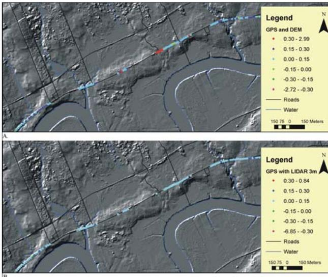
**Figure 4** A. The GPS points colour-coded based on  $\Delta Z$  (GPS-LIDAR DEM) overlaid on the shaded relief LIDAR DEM.
