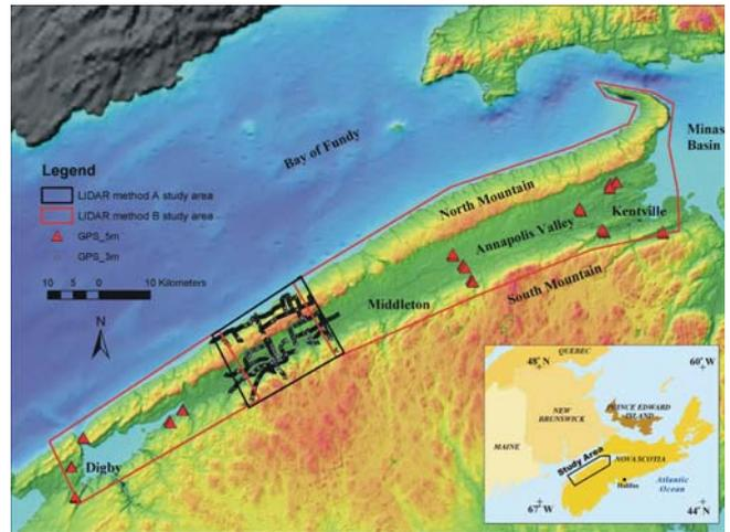
**Figure 1** Colour shaded relief of 20 m DEM for the Annapolis Valley, Nova Scotia, highlighting the study areas of LIDAR methods A and B. Vehicle mounted real time kinematic GPS measurements were used for study area A and static GPS measurements were used for study area B validation. The original 20 m DEM was produced by the Nova Scotia Geomatics Center, Service Nova Scotia & Municipal Relations. Location map inset in lower right shows the study area location in Maritime Canada.
