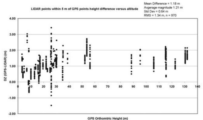
**Figure 8** Graph of  $\Delta Z$  (GPS-LIDAR) of all LIDAR ground points for method B within 5 m of GPS points versus the orthometric height. The mean  $\Delta Z$  is 1.18 m, with an average magnitude of 1.21 m, a standard deviation of 0.64 m and a RMS error of 1.34 m. Note  $\Delta Z$  is denoted as  $DZ$  on the graph.
