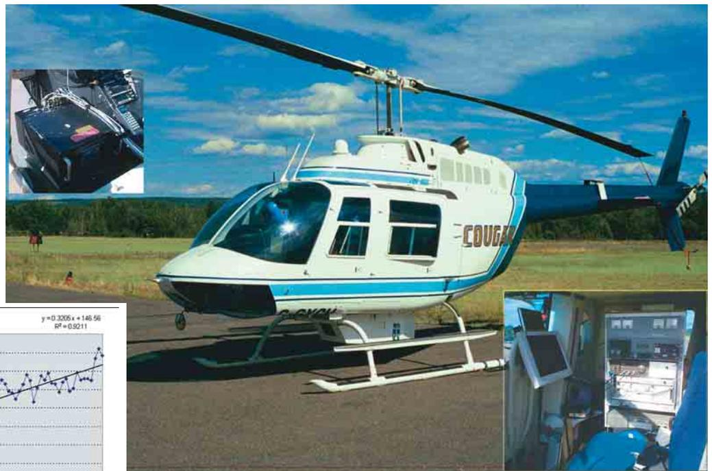
**FIGURE 3** A pod containing the LIDAR and video system was fitted to the belly of this local helicopter. The GPS antenna is located halfway along the tail of the helicopter. The lower right inset shows the LIDAR operator controls. The inset in the upper left shows the inertial reference system used to measure the attitude.
