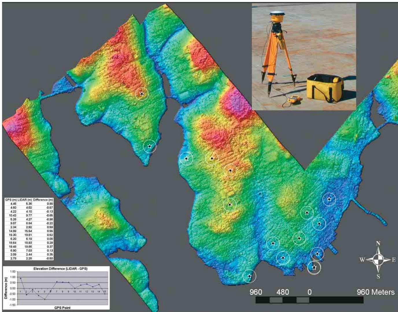
**FIGURE 4** We constructed this bald-Earth DEM from the ground LIDAR hits. GPS validation points (black stars with circles) are overlaid. The table in the lower left (top) shows the differences in orthometric height between the GPS points and the DEM. The graph on the lower left (bottom) indicates an average difference of 4.1 centimeters between GPS points and the LIDAR surface.
