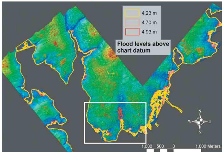
**FIGURE 6** The three modeled flood extents are layered over the color shaded relief image of the LIDAR DSM for Charlottetown (yellow=4.23 meters, orange=4.70 meters, and red=4.93 meters above Chart Datum). The flood modeling was done on the modified bald-Earth DEM; however, the DSM is used to visualize the results. The white box corresponds with the area illustrated in Figure 7.
