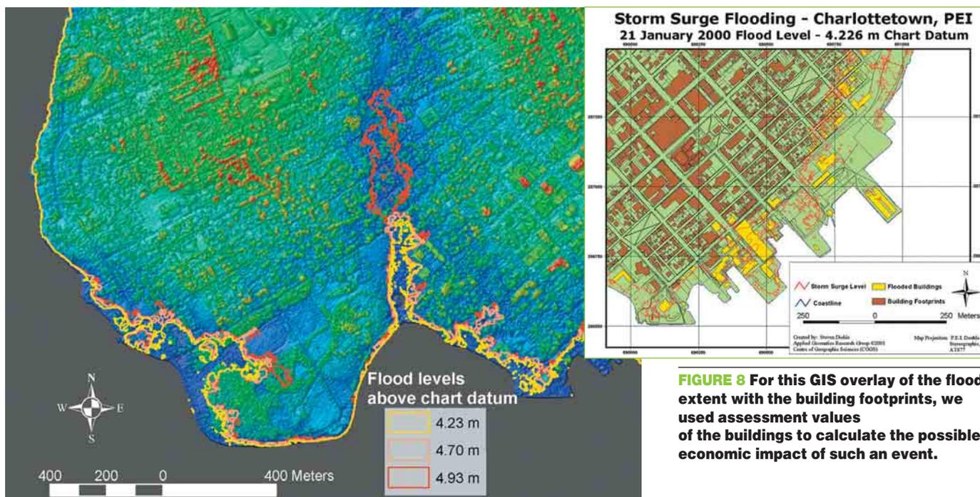
**FIGURE 7** Close-up of the three flood extents for the waterfront area of Charlottetown. The image is a color shaded relief of the DSM.
