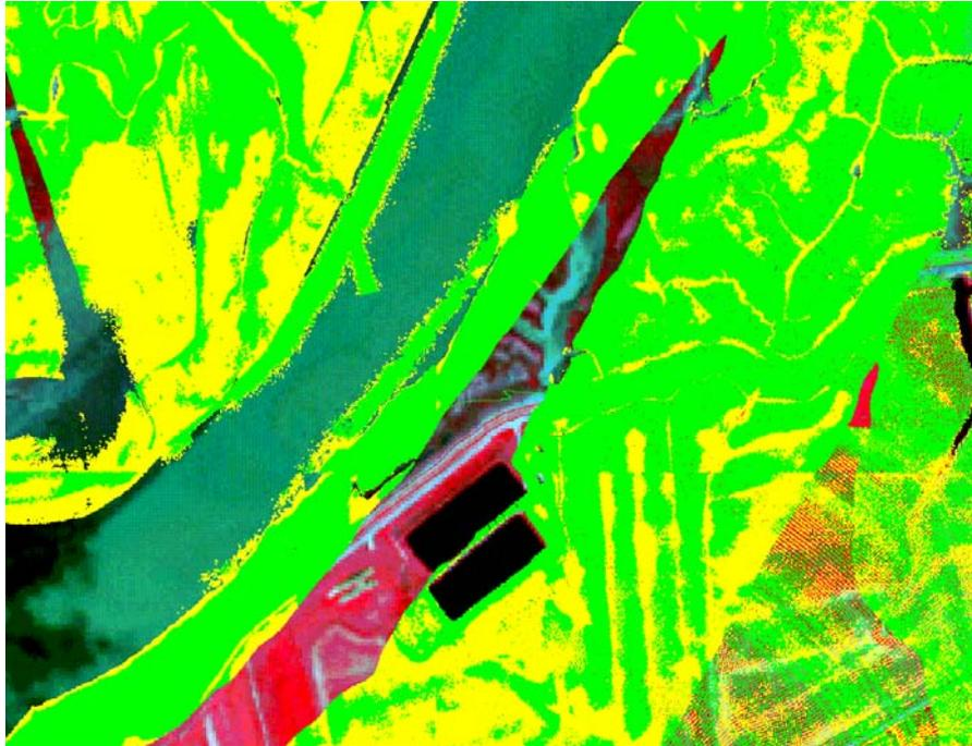
**Figure 15.4 Terra LIDAR points (green=ground, yellow=non-ground) over an Ikonos image for the Grand Pre dyke lands. Notice the missing swaths of data through the centre of the image and to the west. As a result of this missing data the dyke is not represented. Also the classification of ground and non-ground is not correct for the dyke area. Includes material copyright Space Imaging, LCC.**
