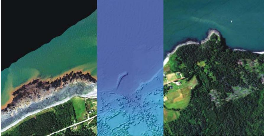
**Figure 15.2** Mosaic of 1 m CASI at low tide (left image), 2 m LIDAR DSM at low tide (centre image), and 3 m CASI at high tide (right image) for Port Lorne along the Bay of Fundy. Overall image is approximately 4 km across.
