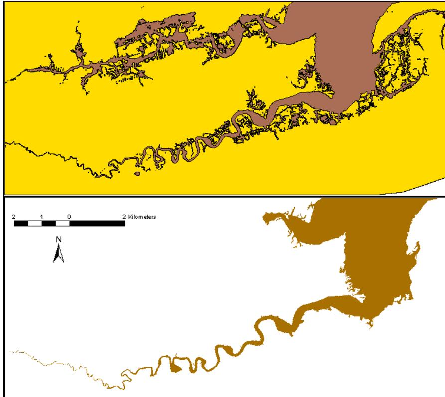
**Figure 15.6** Example of how the flood-risk polygons are generated. Top image is the result of coding all cells less than or equal to 4 m. Bottom image shows only the areas that have connection with the bay or estuary. Flood level is 4 m above MSL, average high tide is 5.9 m above MSL.
