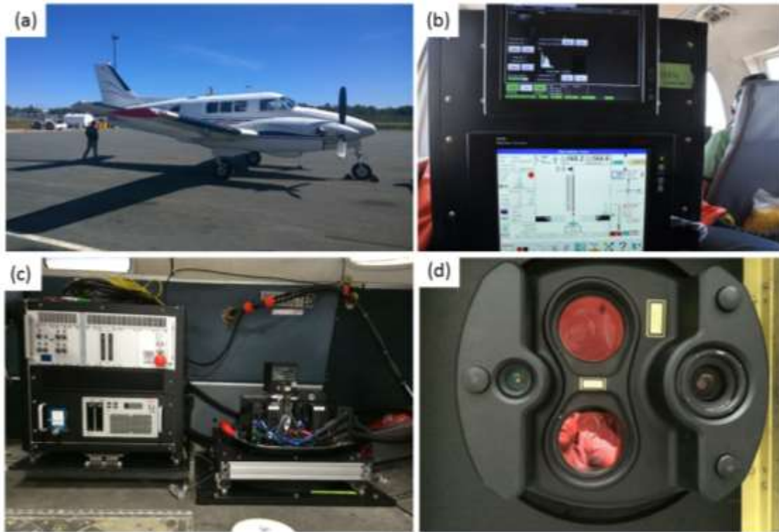
Figure 3 (a) Aircraft used for September 2014 lidar survey; (b) display monitors on a rack as seen by lidar operator in-flight; (c) main body of sensor control rack (left) and lasers and cameras located over the hole cut in the bottom of the plane (right); (d) large red circles are the lasers; the RCD30 lens (right) and low resolution camera (left) as seen from the bottom of the aircraft.
