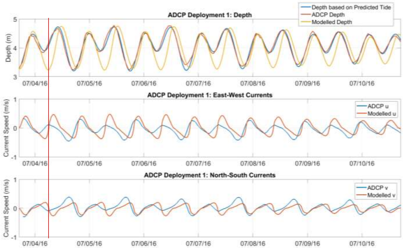
Figure 3.13: Deployment 1 depth and current validation. A -0.6 m offset was applied to the modelled depth, as described in the text (top panel). Current flowing in the East-West direction ( u ) are shown in the middle panel and current flowing in the North-South direction ( v ) are shown in the lower panel. The red line marks a higher low tide when the model over-predicts the tidal amplitude and east-west currents.
