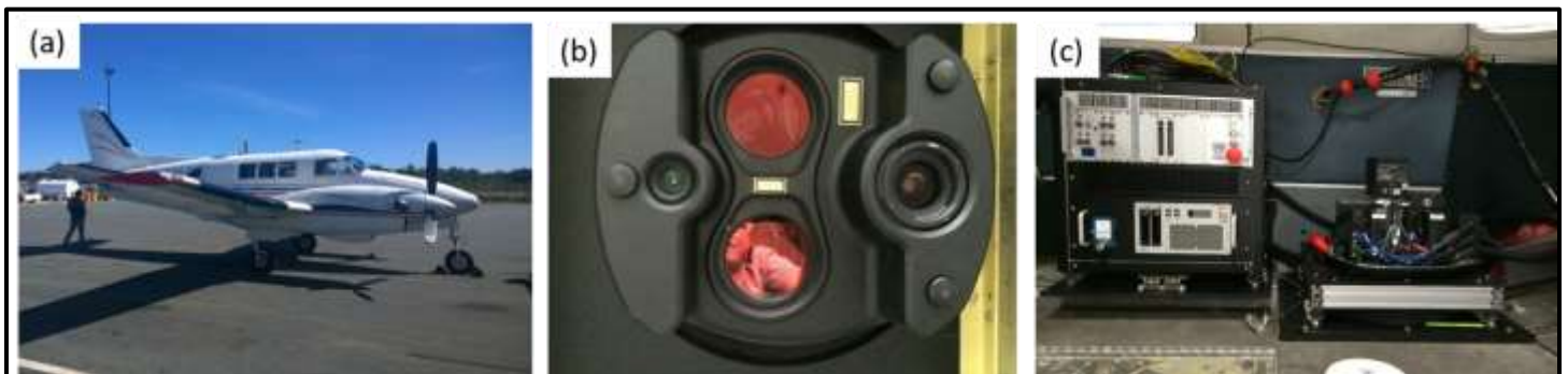
Figure 2.2: (a) Aircraft used for September 2014 lidar survey; (b) large red circles are the lasers; the RCD30 lens (right) and low resolution camera (left); (c) main body of sensor (left) and laser pointing through a hole cut in the bottom of the plane (right).
