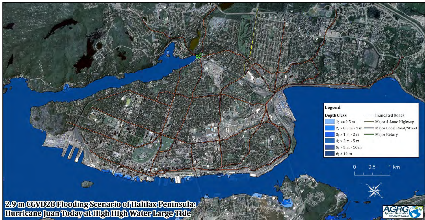
Figure 7. The flooding extent and depth of flooding of the Halifax Peninsula under a 2.9 m flooding scenario, representing a Hurricane Juan event today occurring at high high water large tide.
