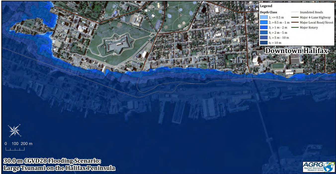
Figure 11. The flooding extent and depth of downtown Halifax under a 30.0 m flooding scenario, representing a large tsunami hitting the peninsula.
