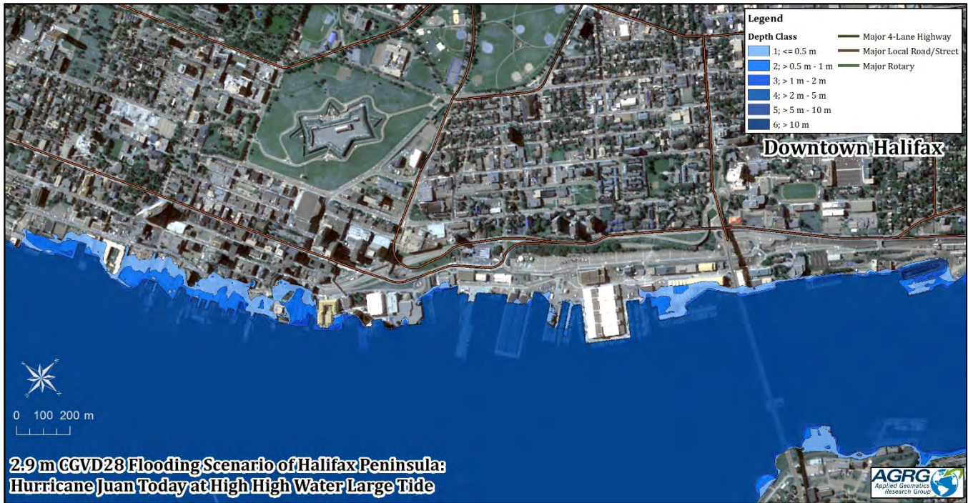
Figure 8. The flooding extent and depth of flooding of downtown Halifax under a 2.9 m flooding scenario, representing a Hurricane Juan event today occurring at high high water large tide.
