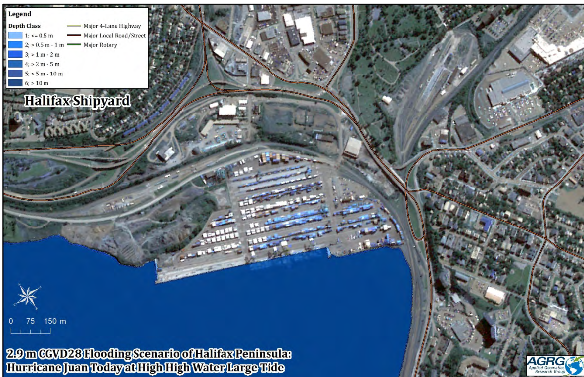
Figure 9. The flooding extent and depth of flooding of the Halifax Shipyard under a 2.9 m flooding scenario, representing a Hurricane Juan event today occurring at high high water large tide.
