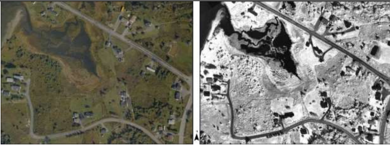
Figure 12 Example of RGB image on the left and grey scale near infrared band on right.
