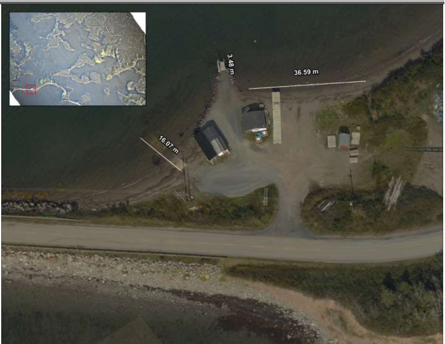
Figure 13 Example of RCD30 orthophoto 5 cm mosaic where measurements of boat launch sites can be made directly from the orthophoto.
