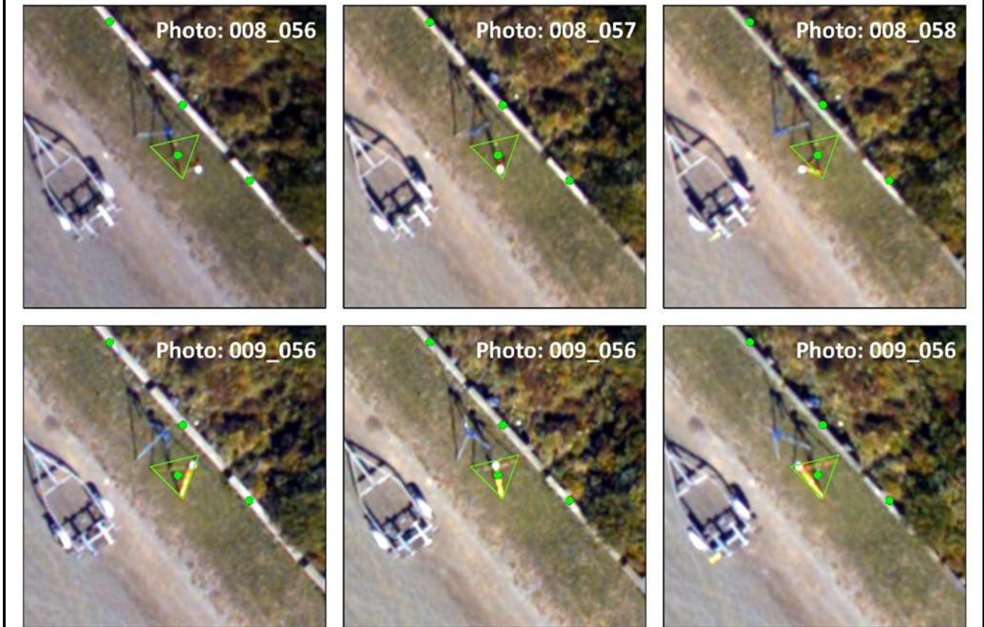
Figure 12 Example of multiple frames (56, 57, and 58) from multiple flight lines (008 on top and 009 below) of the GPS base station location at Little Harbour after orthorectification. The green dots are GPS locations along the parking lot rail and the aircraft control benchmark on the ground below the tripod where the bottom of the legs are represented by the green diamond.
