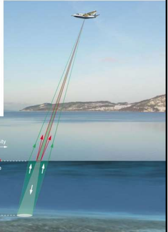
Figure 2 Principals of topo-bathymetric lidar. The system utilizes two lasers, a near infrared and a green laser to surface the land and marine topography.
