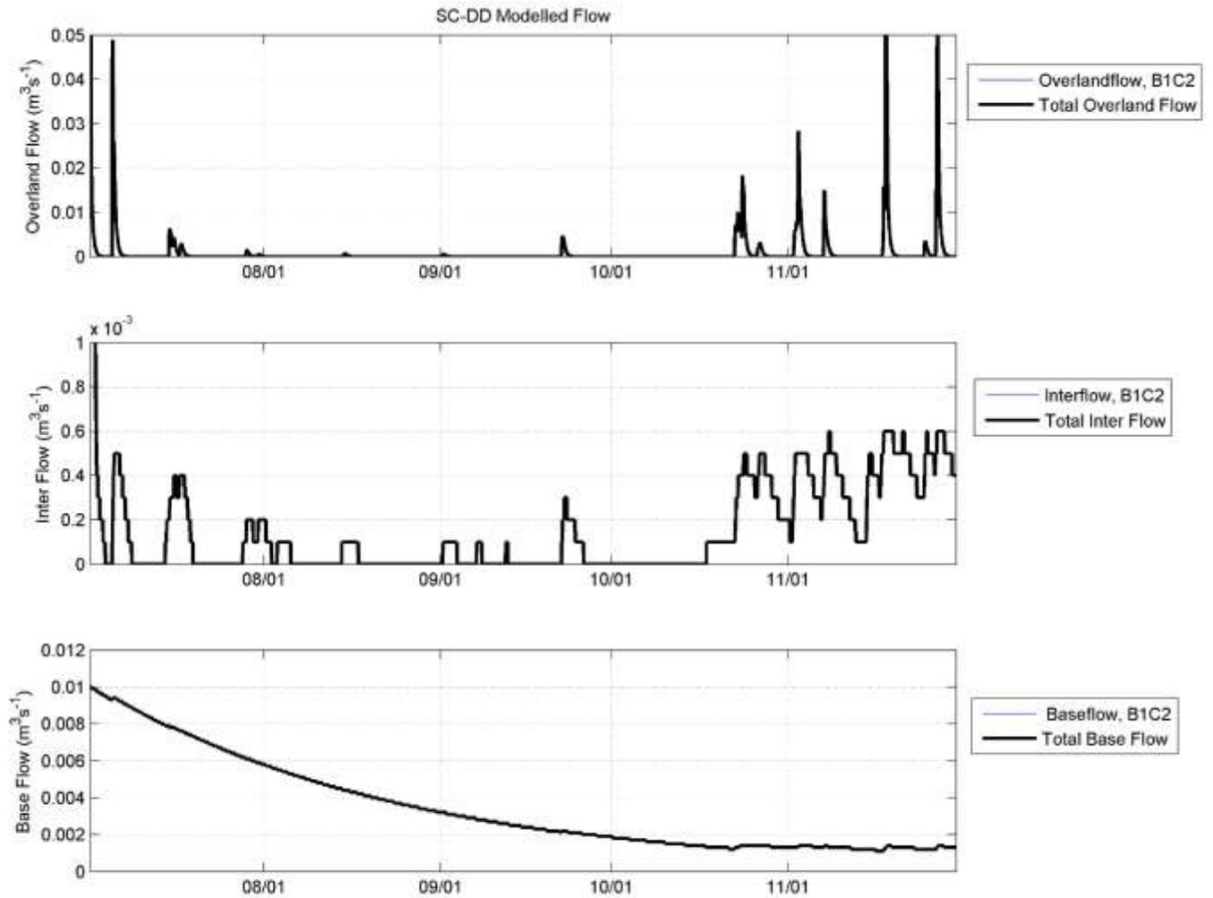
Figure 7.4: Modelled overland, inter, and base flow for the SC-DD between May 15 and November 30, 2014.
