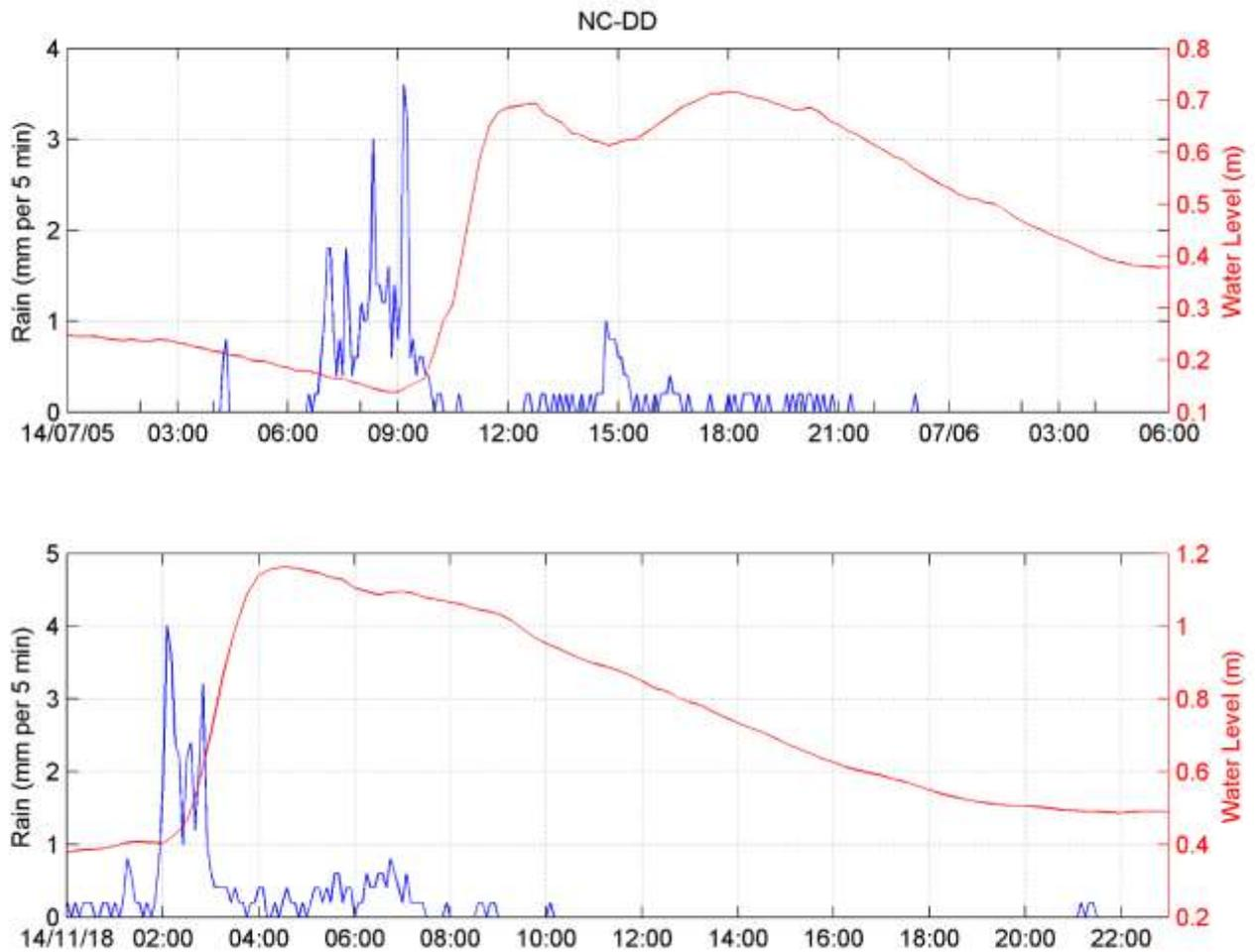
Figure 2.7: Lag at NC-DD between precipitation (as observed at 5 minute sampling interval) and water level on July 5, 2014 (top) and on November 18, 2014. During July when the ground was drier, the lag was ~8-10 hours; in November when the ground was likely much wetter the lag is closer to ~3 hours.
