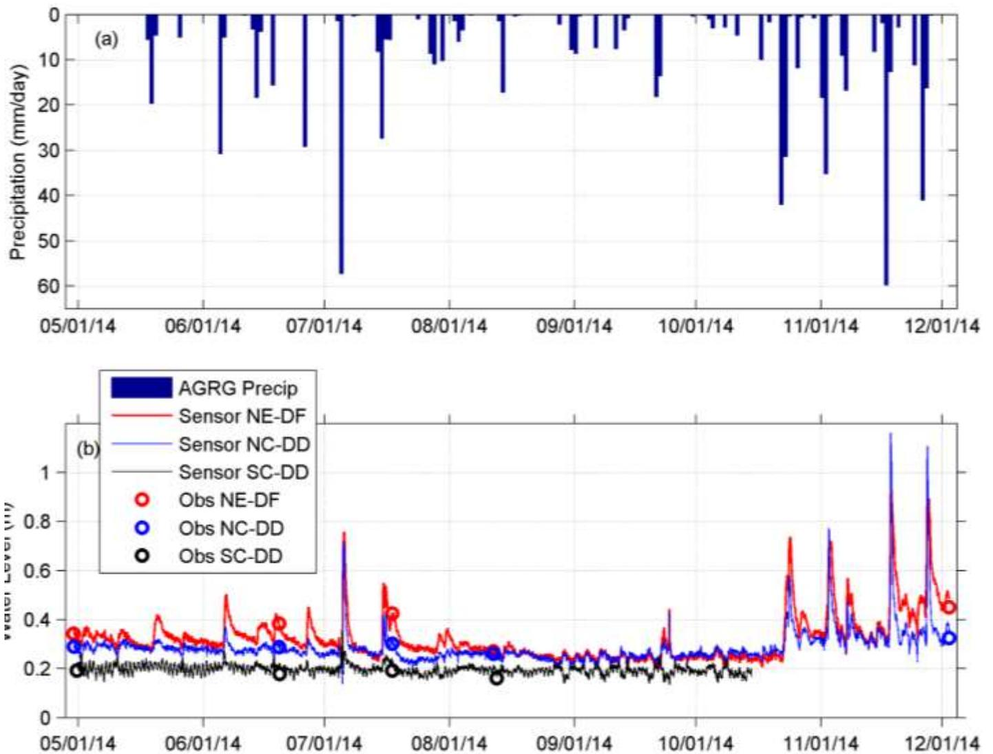
Figure 2.5: (a) Daily precipitation; (b) water level at each of the three sensors as recorded by the sensors, with observed water levels shown as circles.
