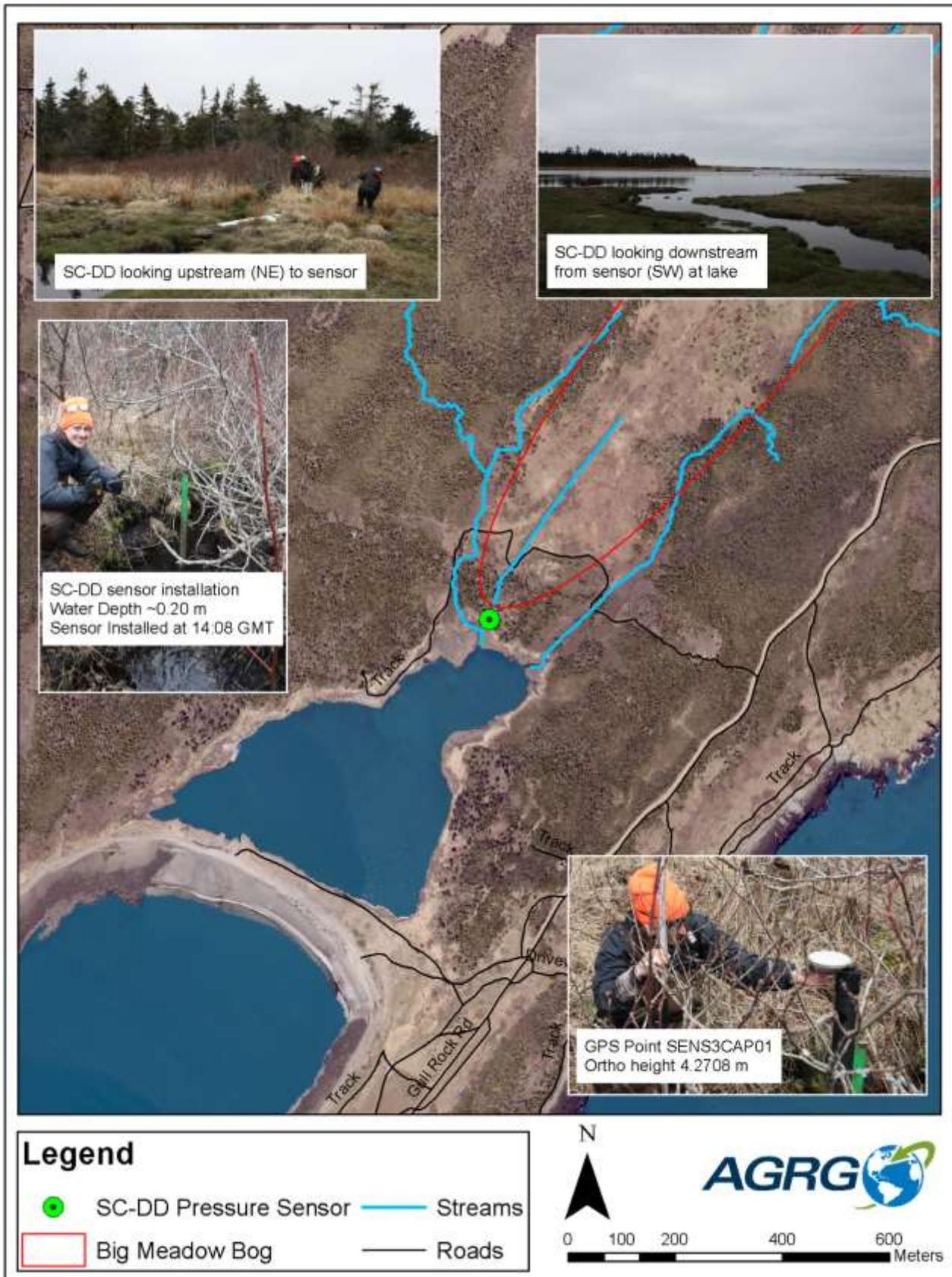
Figure 2.4: SC-DD map and installation photos and notes.
