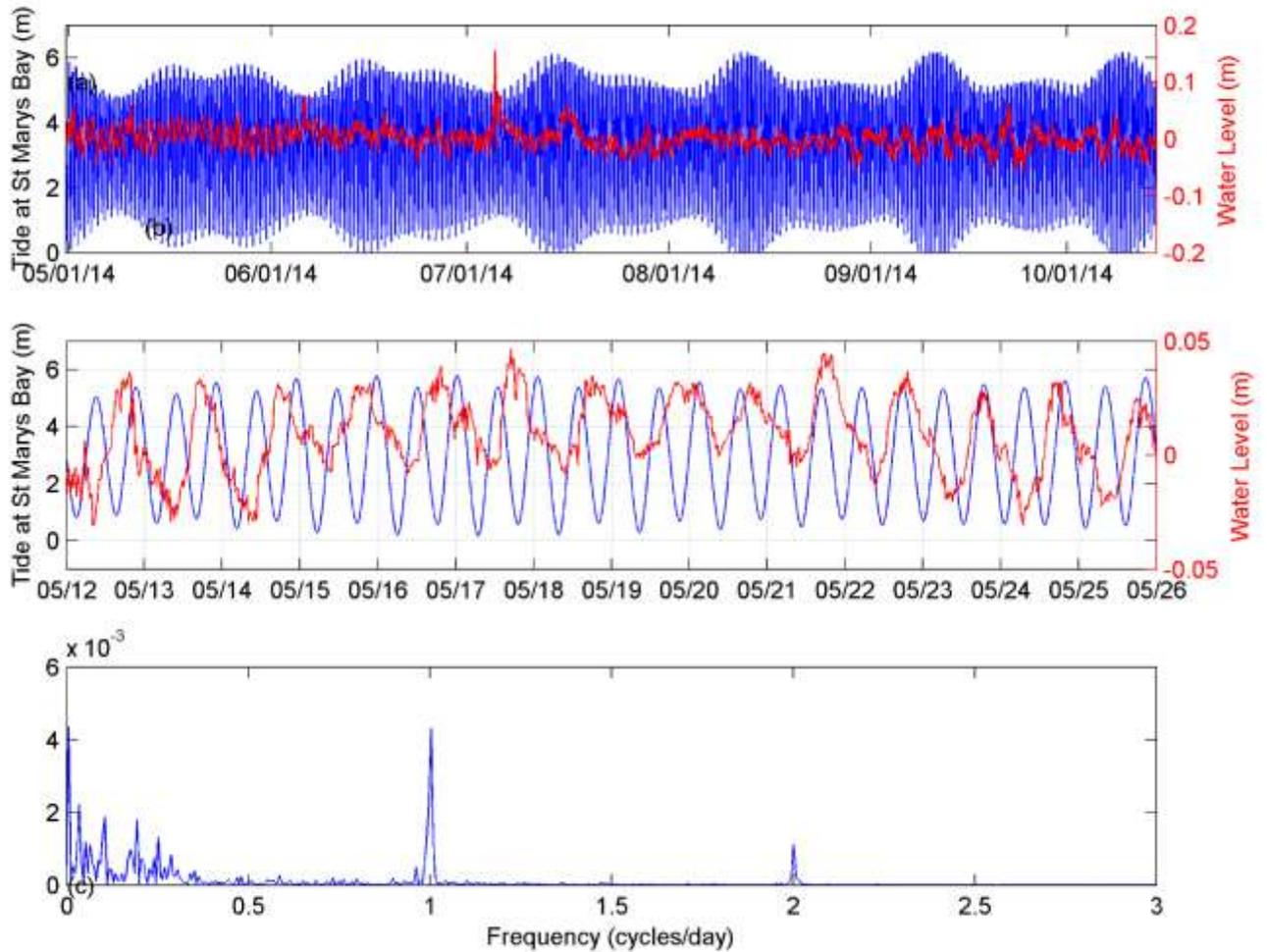
Figure 2.9: Predicted tide at St Mary's Bay, NS, and normalized water level (mean removed) measured by the sensor at SC-DD for (a) the entire deployment and (b) a two-week period; (c) shows a frequency analysis of the normalized water level with peaks at one and two cycles per day.
