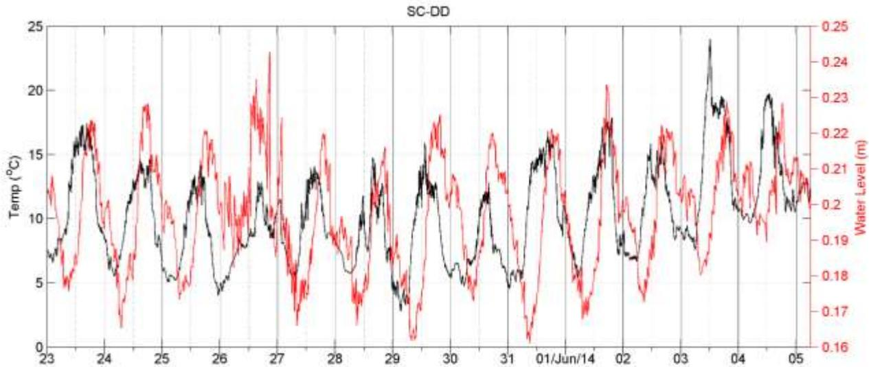
**Figure 2.10: Temperature and water level at SC-DD. Water level increases following the daily temperature peak.**
