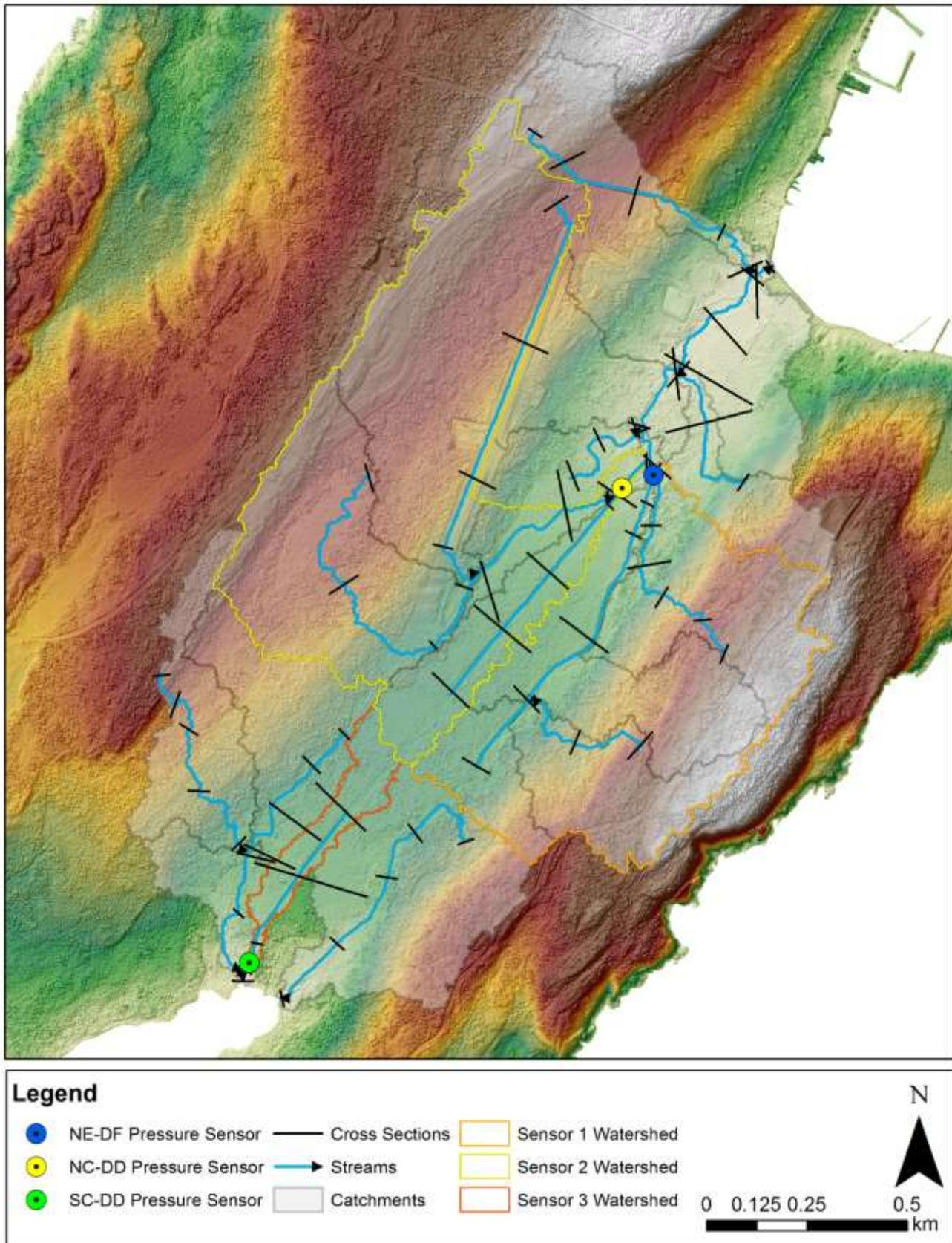
Figure 2.13: Digital elevation model of Brier Island showing the three pressure sensors, watersheds and catchment areas, stream branches and the cross-sections used in the 1-D hydrodynamic model.
