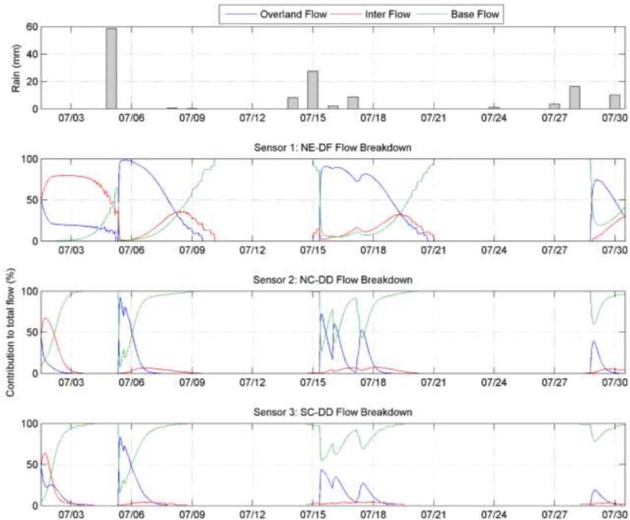
Figure 3.5: Contribution of overland, inter and base flow to total flow at each sensor location during July 2014.
