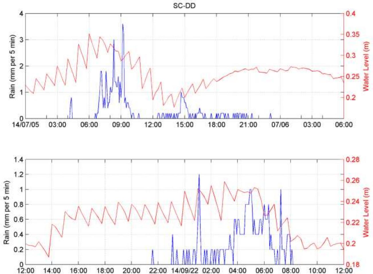
Figure 2.8: Lag at SC-DD between precipitation (as observed at 5 minute sampling interval) and water level on July 5, 2014 (top) and on September 21 and 22, 2014. We see almost no lag during either time frame.
