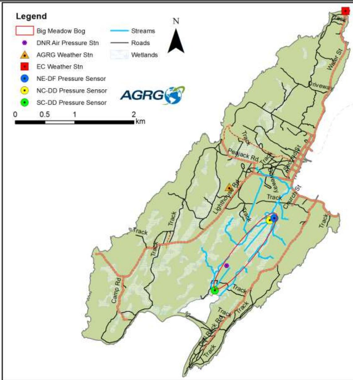
Figure 2.1: Map showing the three pressure sensors and two meteorological stations used for this study.
