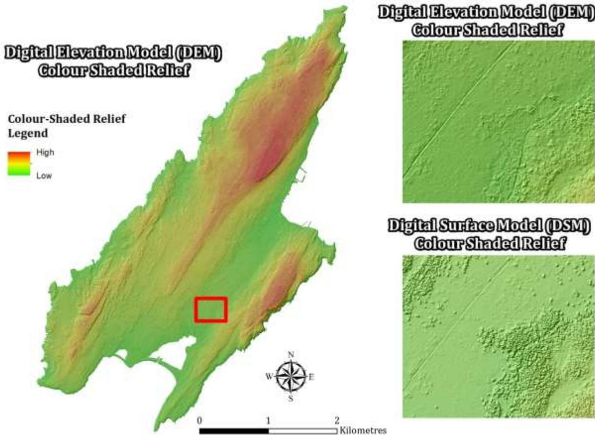
Figure 2.12: Colour shaded relief maps of the 2006 LiDAR derived 1 m digital elevation and surface models of Brier Island from MacDonald and Webster (2014).
