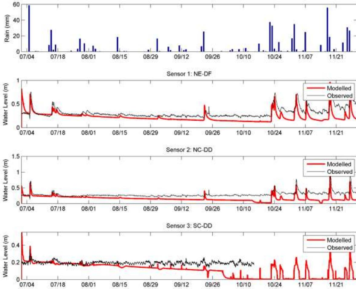
Figure 7.1: Water level calibration plot for July 1 – Nov. 30, 2014.
