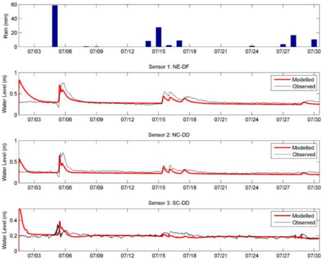
Figure 2.16: Precipitation (top); modelled and observed water level at each sensor location during July 2014.
