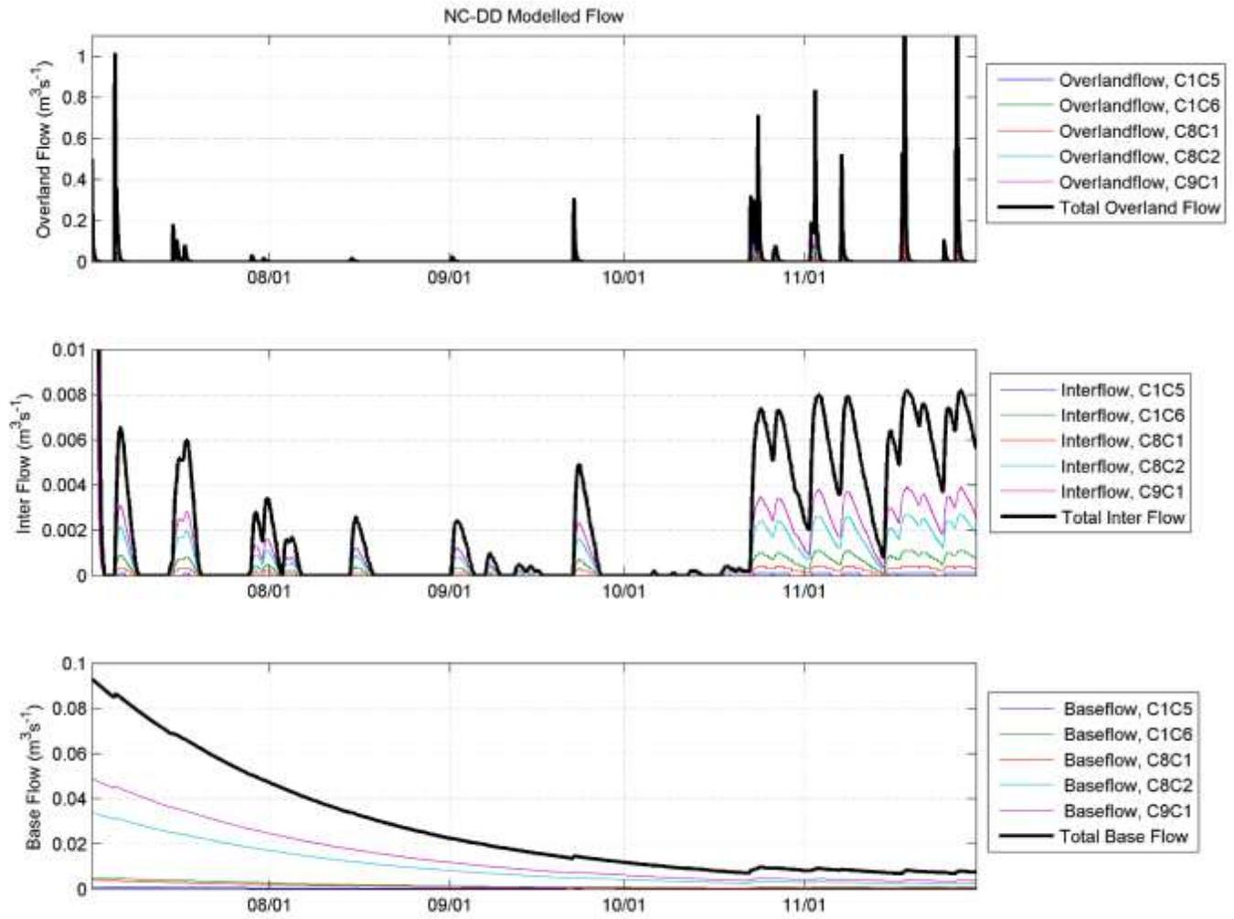
Figure 7.3 Modelled overland, inter, and base flow for the NC-DD between May 15 and November 30, 2014.
