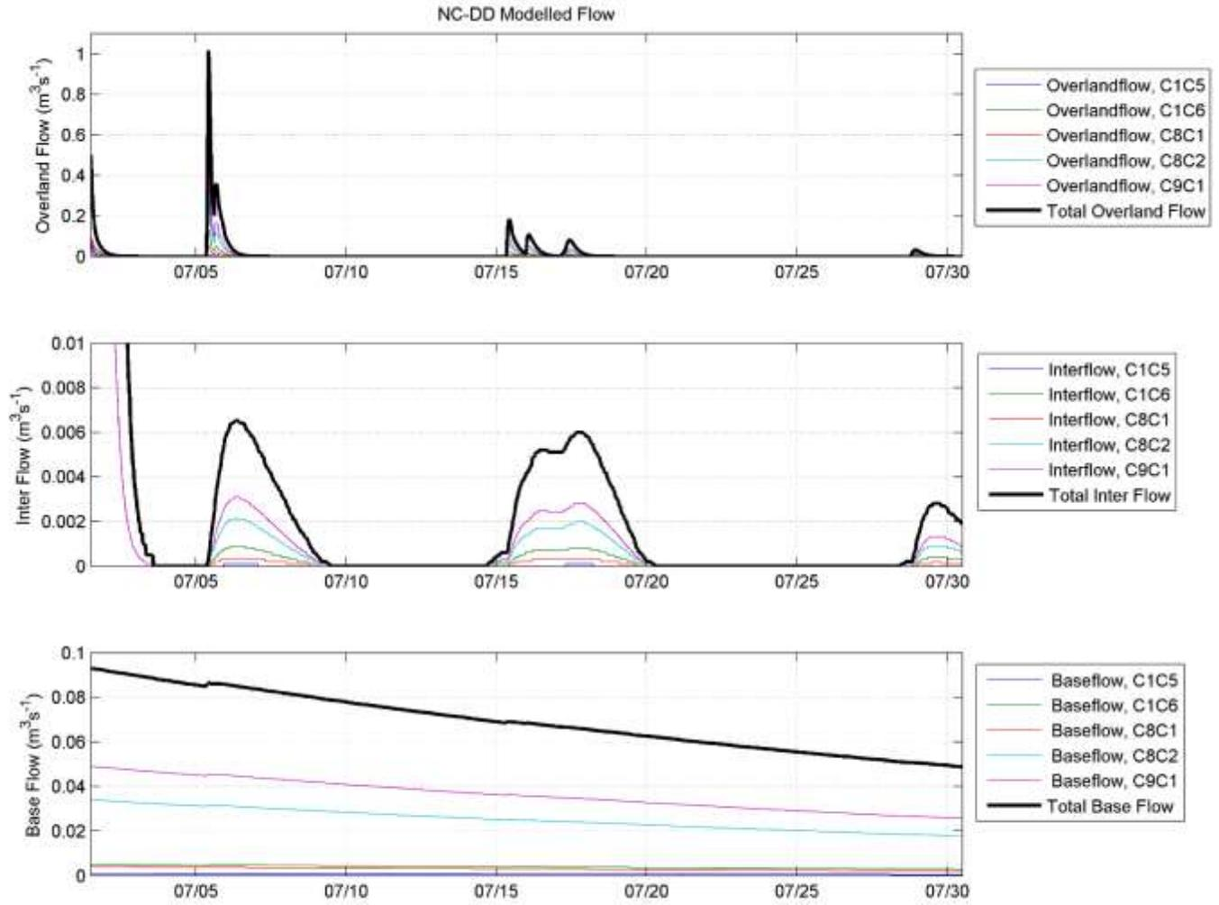
Figure 3.3: Modelled overland, inter, and base flow for the NC-DD during July 2014.
