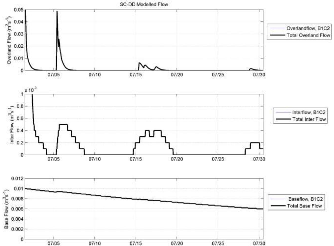
**Figure 3.4: Modelled overland, inter, and base flow for the SC-DD during July 2014.**
