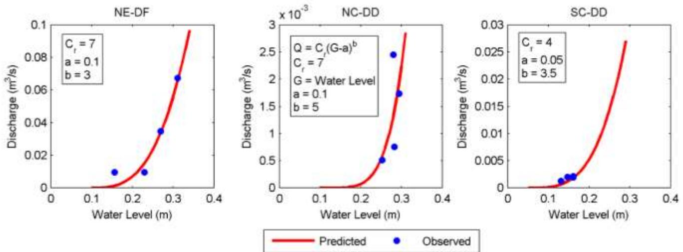
Figure 2.15: Rating curves derived from measured water level and discharge at each sensor. Note the different scale of the y-axis in each panel showing the differences in discharge at each location.
