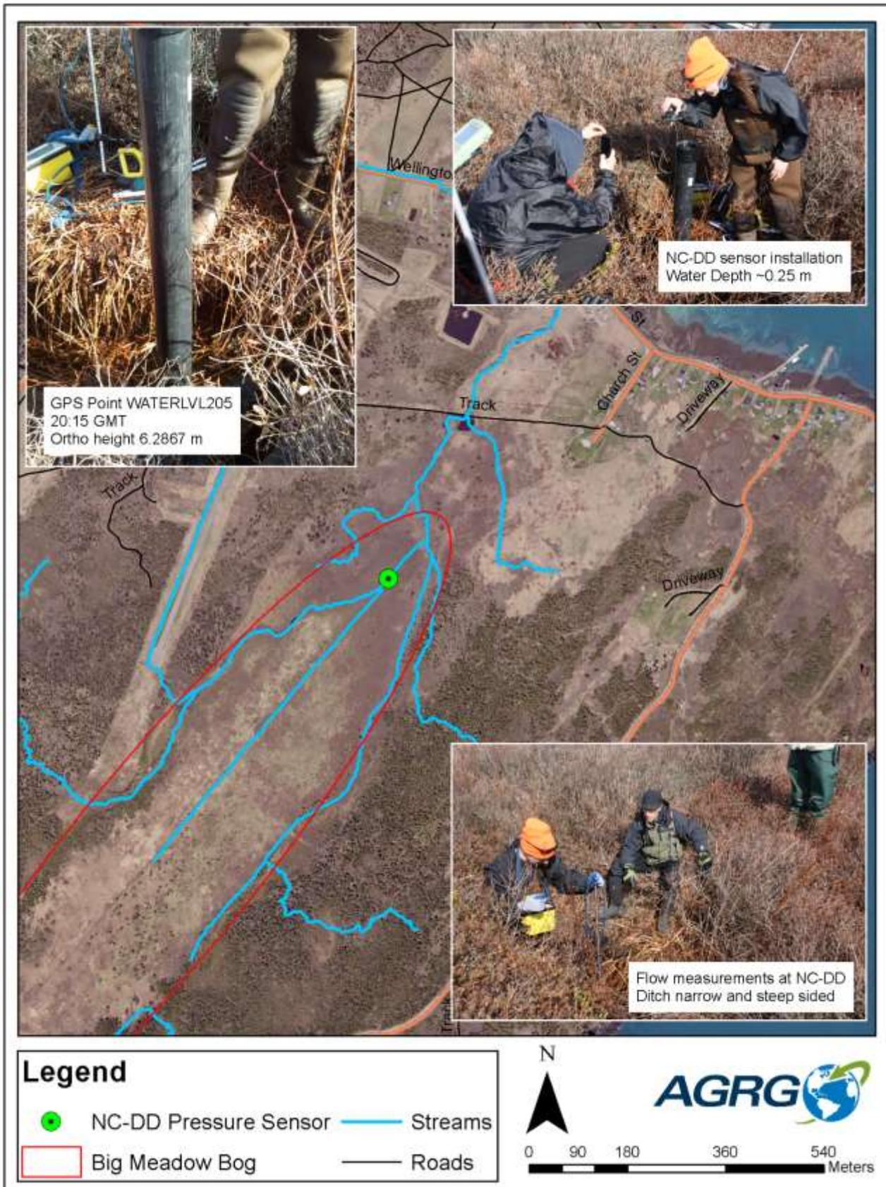
Figure 2.3: NC-DD map and installation photos and notes.
