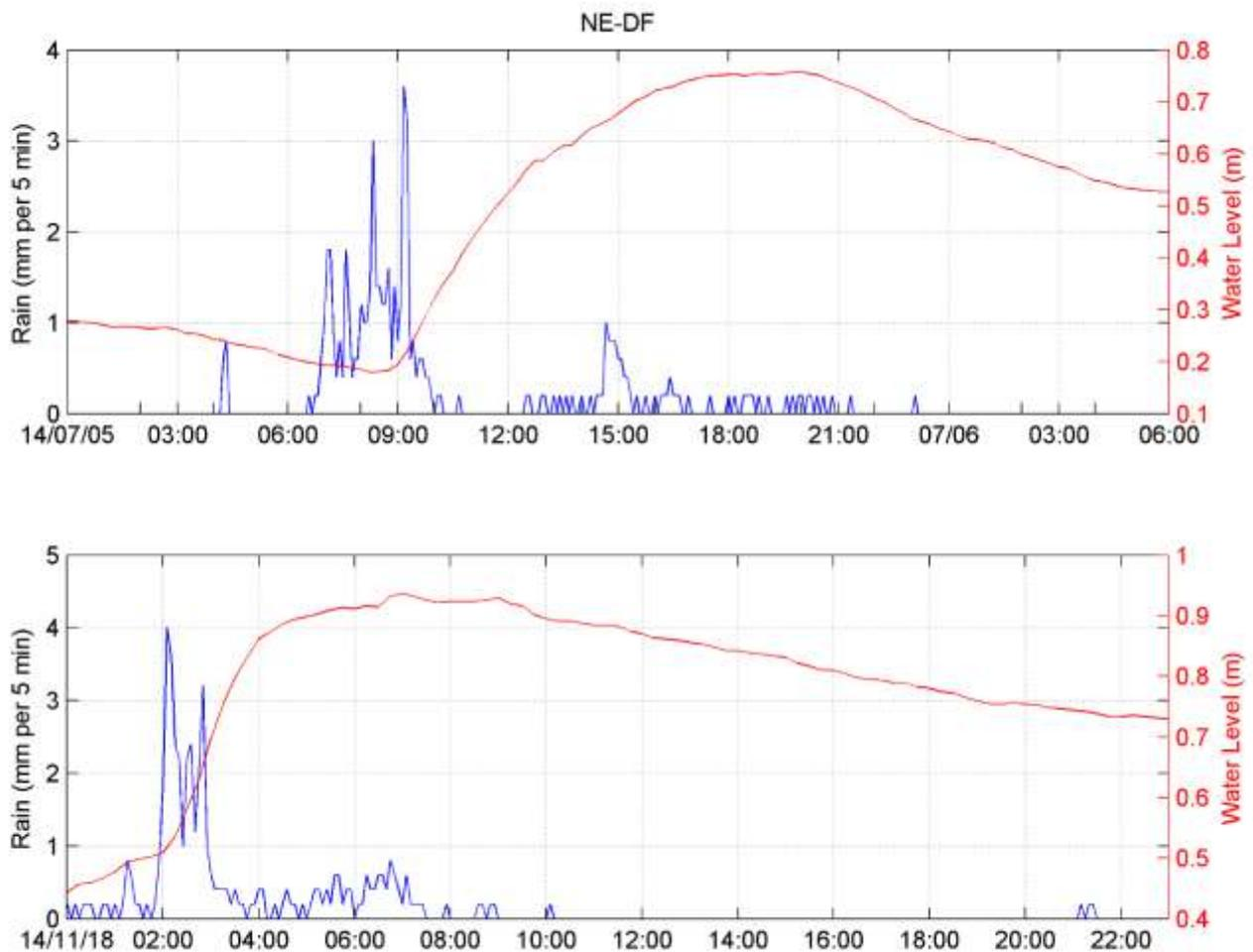
Figure 2.6: Lag at NE-DF between precipitation (as observed at 5 minute sampling interval) and water level on July 5, 2014 (top) and on November 18, 2014. During July when the ground was drier, the lag was ~10-12 hours; in November when the ground was likely much wetter the lag is closer to ~6 hours.
