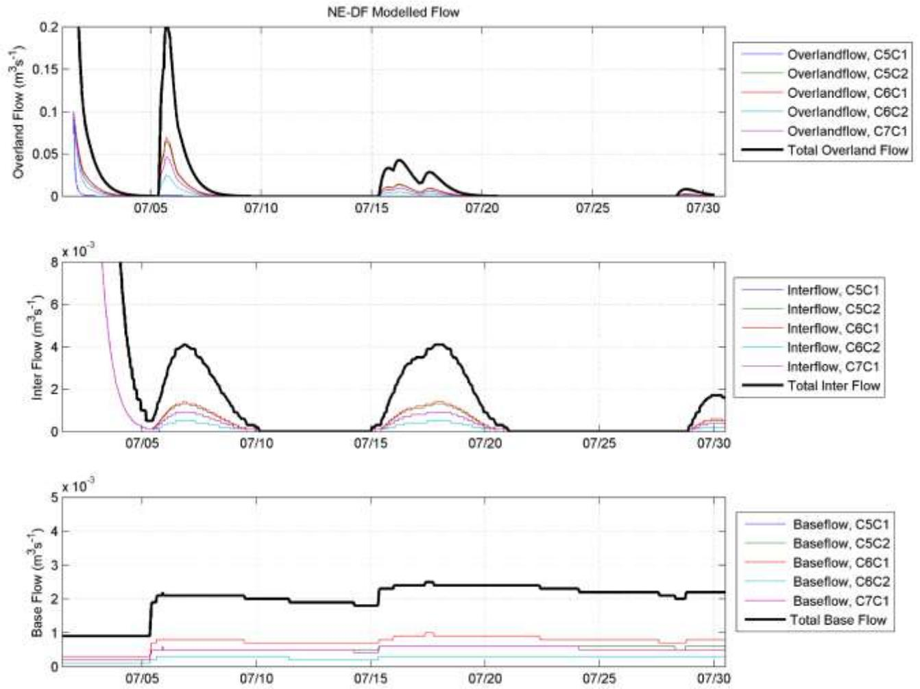
Figure 3.2: Modelled overland, inter, and base flow for the NE-DF during July 2014.
