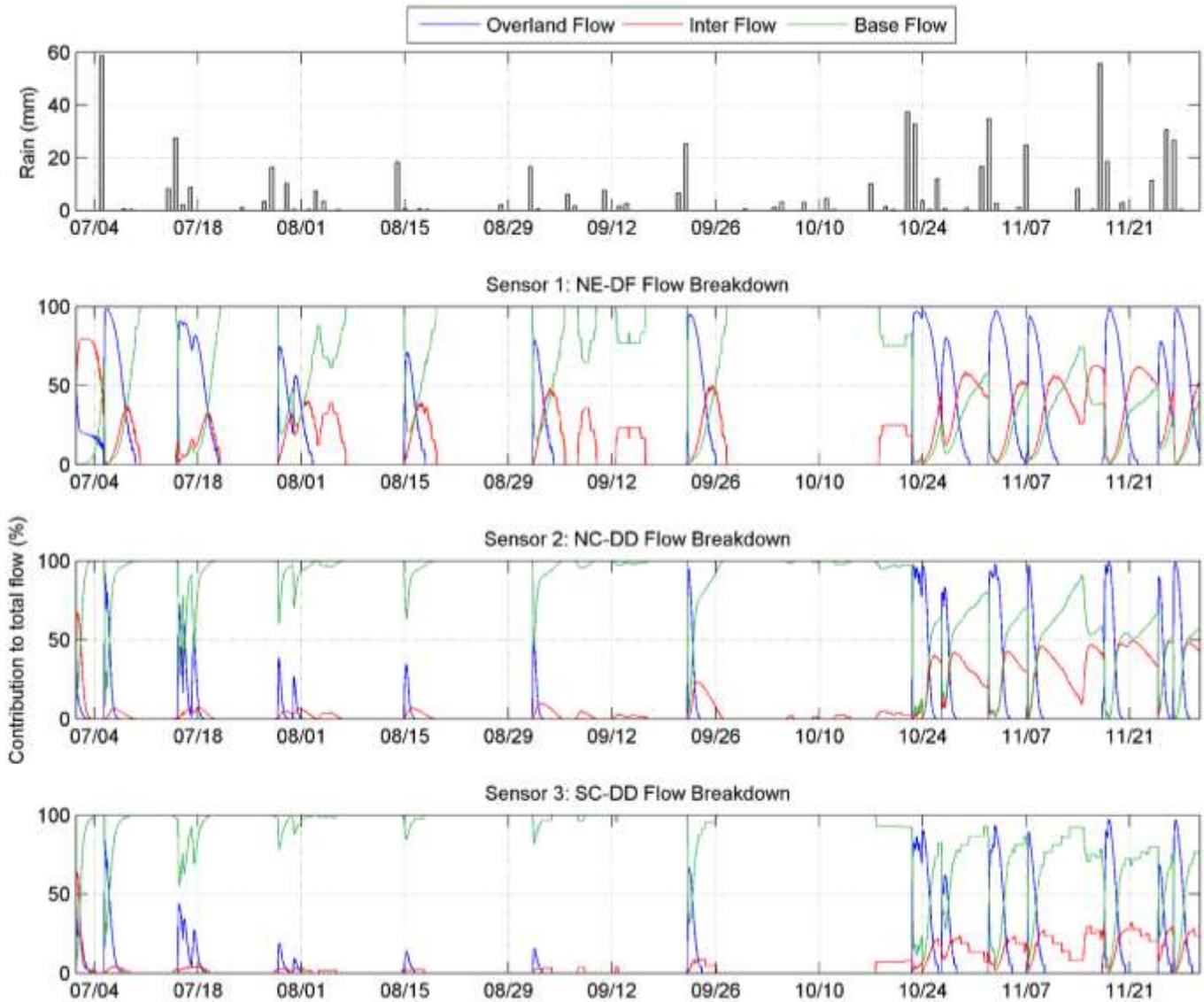
Figure 7.5: Contribution of overland, inter and base flow to total flow at each sensor location between May 15 and Nov. 30, 2014.
