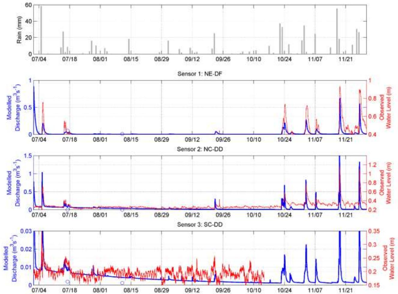
Figure 2.18 Precipitation (top panel); modelled discharge (left axis, blue) and observed water level (right axis, red) between July 1 and Nov 30. Blue circles denote field observations of discharge. Note the different y-axis scales for each subplot.
