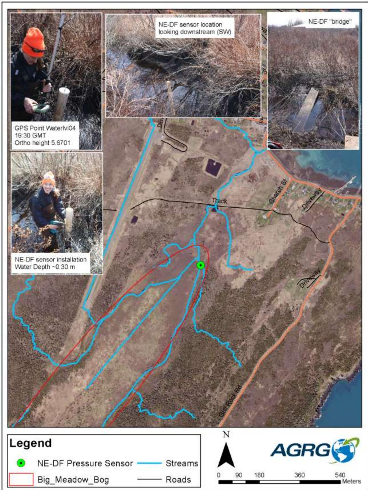
Figure 2.2: NE-DF sensor map and installation photos and notes.
