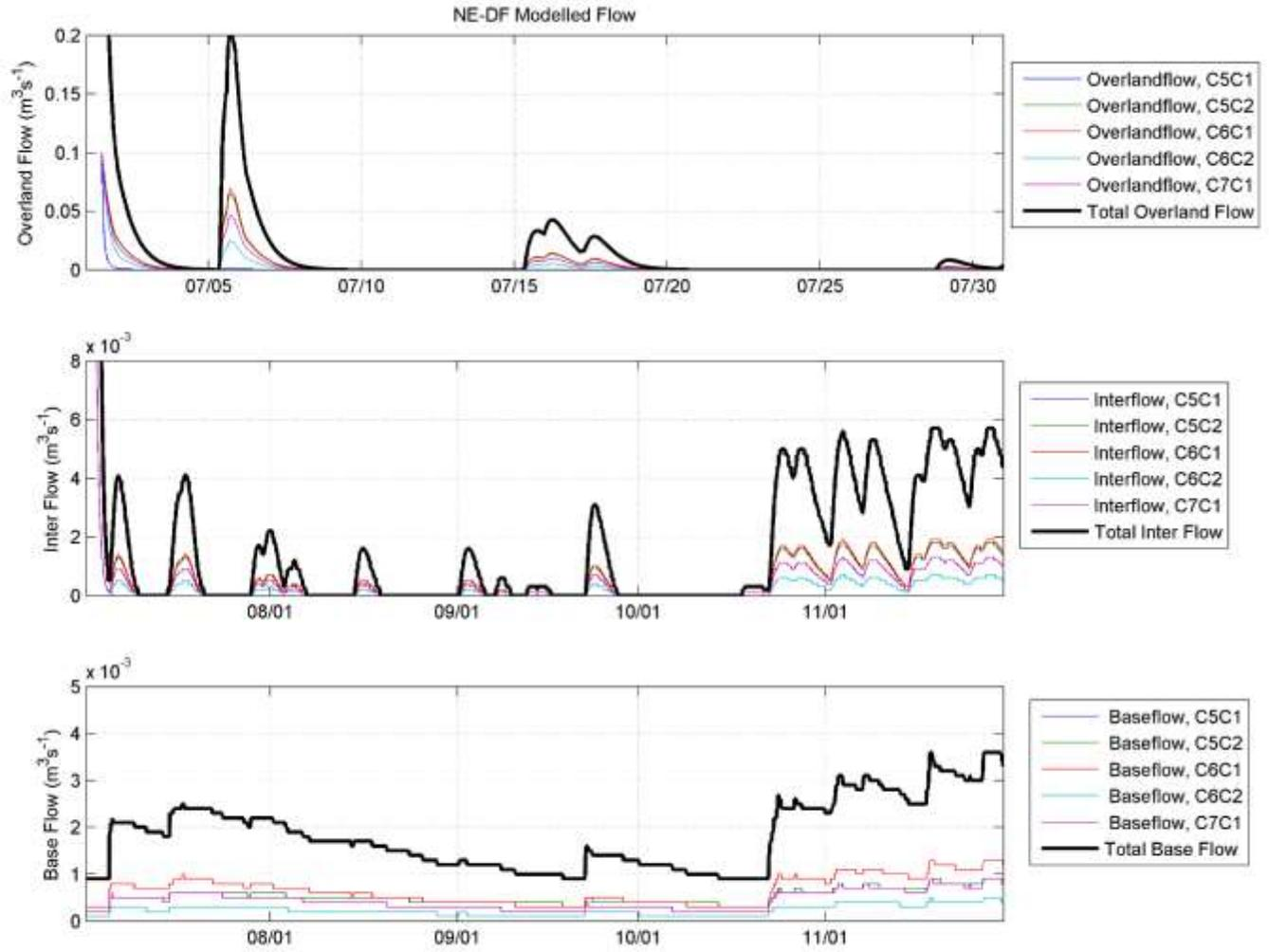
Figure 7.2: Modelled overland, inter, and base flow for the NE-DF between July 1 and November 30, 2014.
