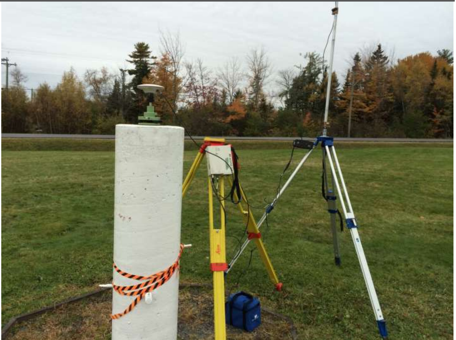
Figure 2 GPS base station used for RTK GPS surveys Oct. 22-23, 2015.
