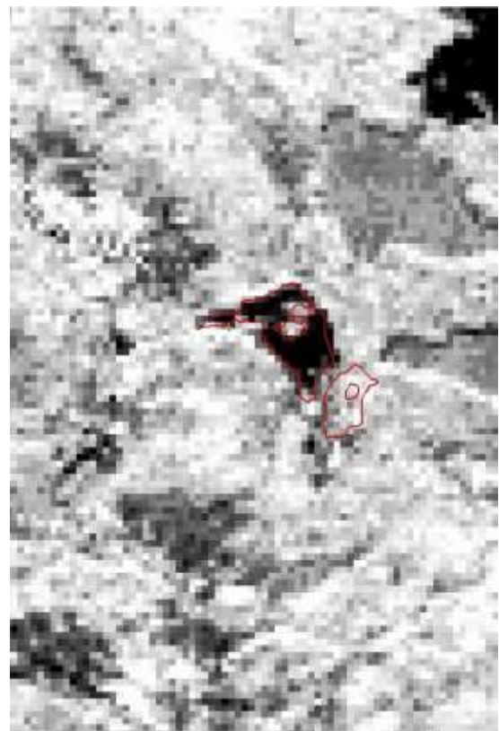
Figure 8: Result of image subtraction of radiometrically corrected imagery. More mid-range grey values represented making dominant change distinction more difficult.
