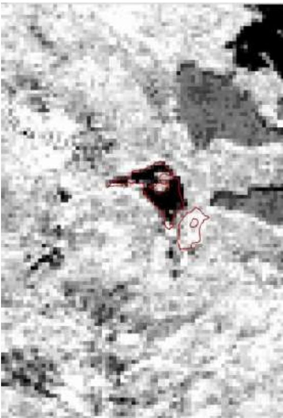
Figure 7: Result of image subtraction of non-radiometrically corrected imagery. Very dark and very light pixels represent drastic change. This dominant change is more distinguishable from moderate change.
