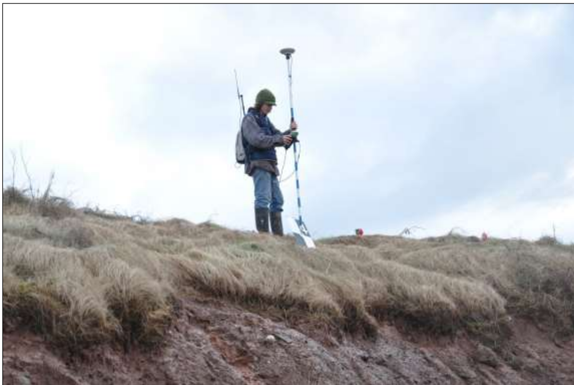
Figure 3 Example of a georeferencing target and GPS positional measurement (precise of 2 cm in Z). The targets are then located in the point cloud and (Fig. 4) and used as control points with the GPS coordinates. A first order polynomial transformation is used to convert the point cloud data to UTM NAD83 zone 20 horizontal coordinates and the elevations are referenced to CGVD28.
