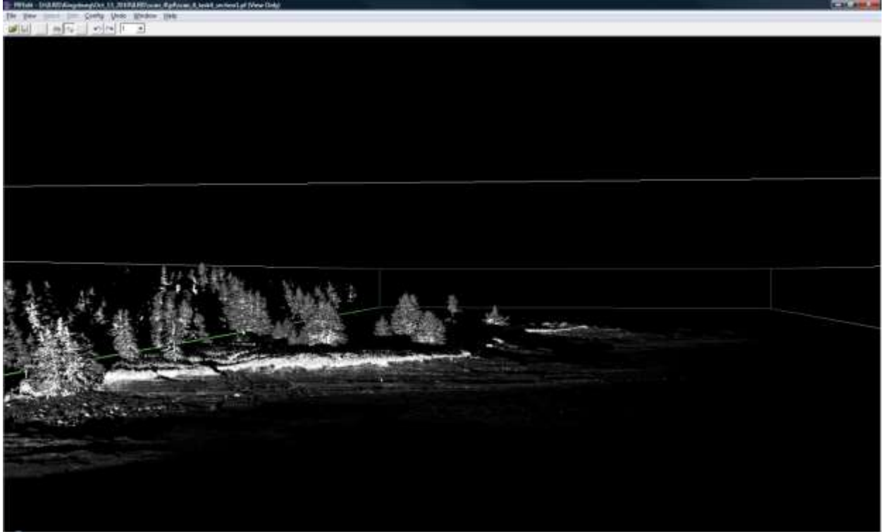
Figure 48 Low relief bedrock point laser scan at Kingsburg.
