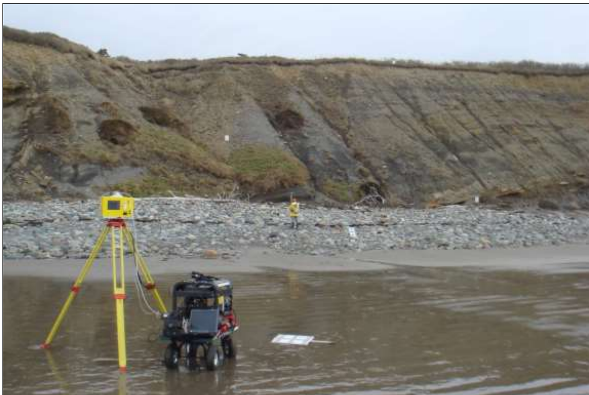
Figure 30 Photo of ILRIS setup for scanning the glacial till bank. Scan represented in Fig. 32 of this area.
