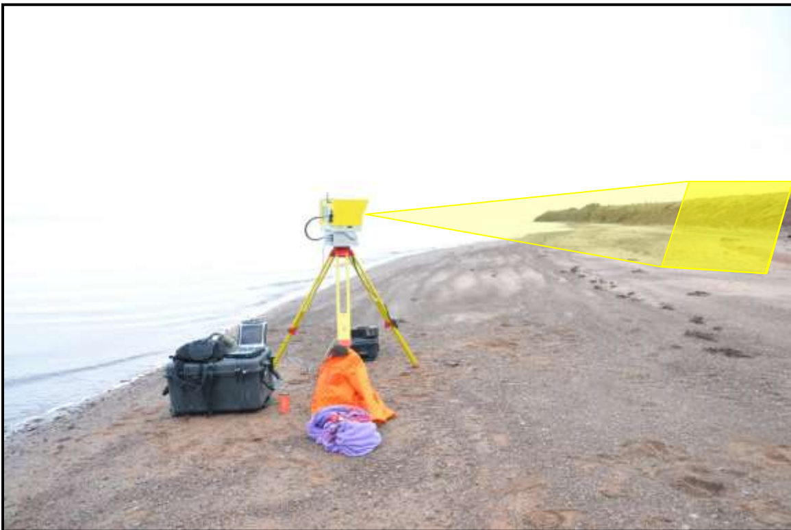
Figure 2 Typical ILRIS setup along the coast. The yellow shaded area is a cartoon to represent the 40 degree by 40 degree field of view.
