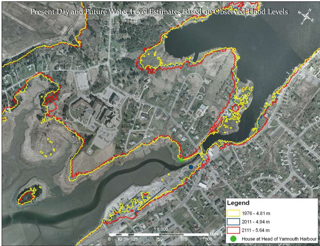
Figure 30 Yarmouth location map. Green dot is the back door step high-water mark and the blue dot is the top of car tire high-water mark RTK-GPS survey locations. The yellow line is the flood limit of 4.81 m high-water (door step elevation), the other lines represent sea-level rise in the future.
