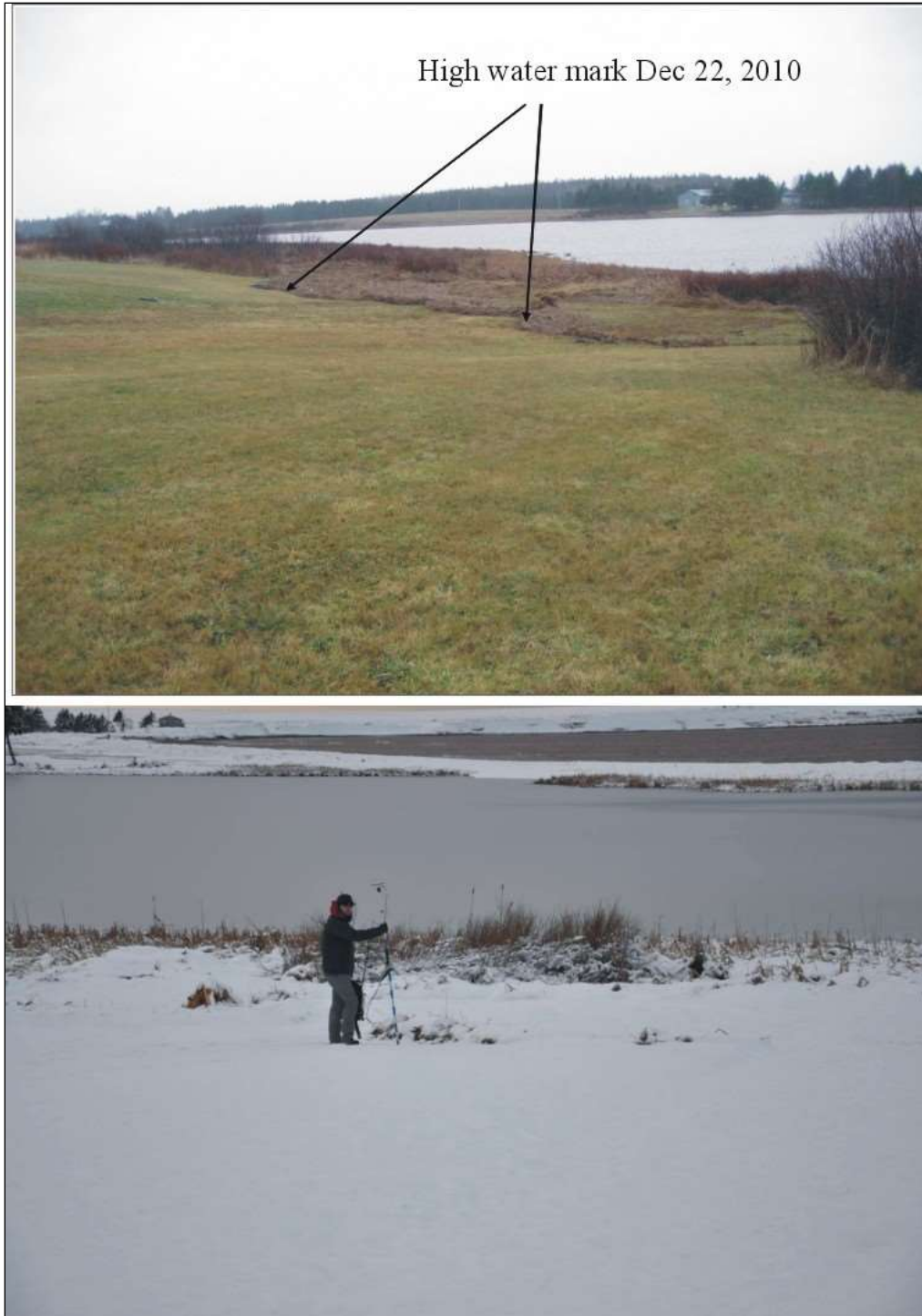
Figure 31 Debris high-water line from Dec 21-22, 2010 storm at Cape John (top photo). RTK GPS of high-water line indicates a water level of 2.38 m CGVD28.
