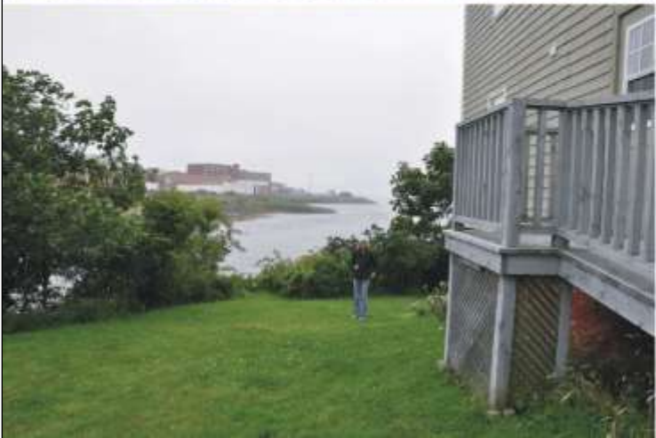
Figure 28 High-water mark being surveyed in Yarmouth from Feb. 3, 1976 Groundhog Day Storm. 4.81 m CGVD28 elevation from GPS of high-water mark.
