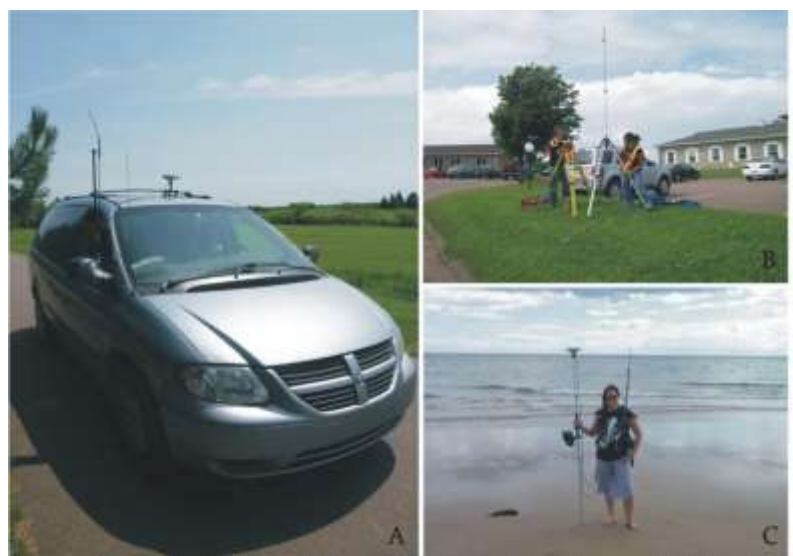
Figure 1. Equipment setup. (A) van RTK setup, (B) setting up a base station over HPN027, and (C) Collecting RTK GPS beach transect.
