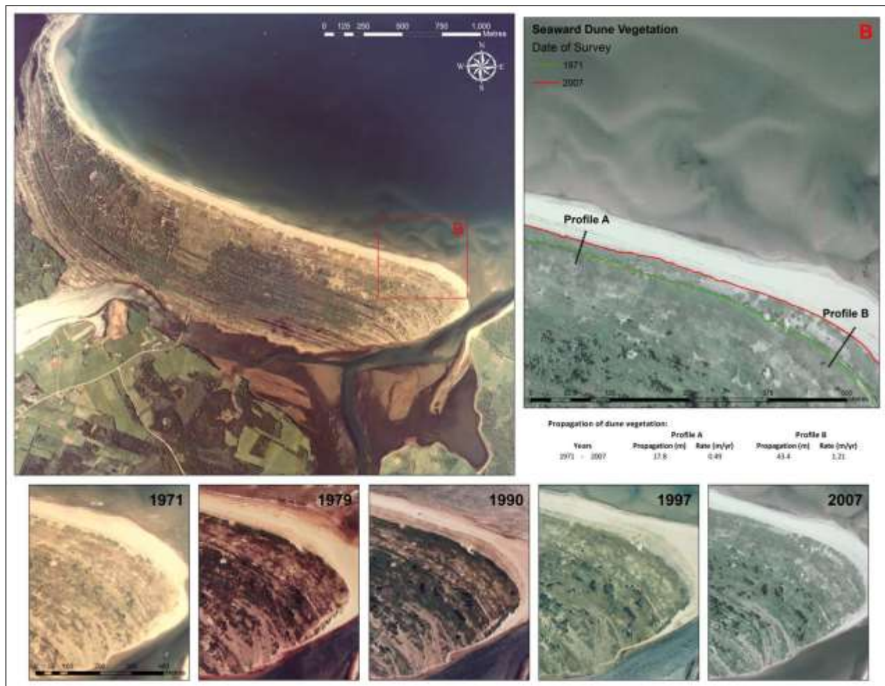
Figure 18 Pomquet Beach detailed coastline change detection. Photos range in time from 1971 to 2007. Coastline in this area has undergone a seaward dune migration over the surveyed dates.
